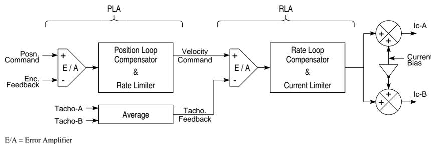
Figure 20.3: Rate loop amplifier.
