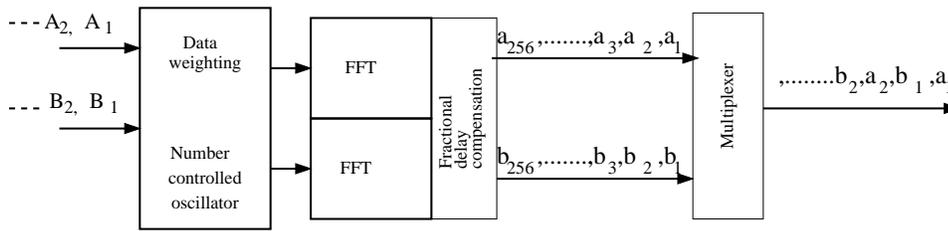
Figure 25.4: Block diagram of the FFT unit of the GMRT correlator
