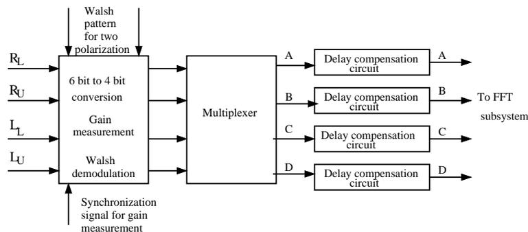
Figure 25.3: Block diagram of the delay-DPC unit of the GMRT correlator
