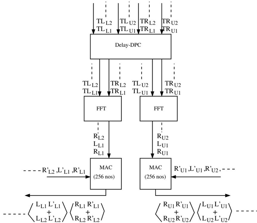
Figure 25.7: Signal flow in the GMRT correlator when it is configured in Indian-Polar mode. See the caption of Figure 25.6 for other details.
