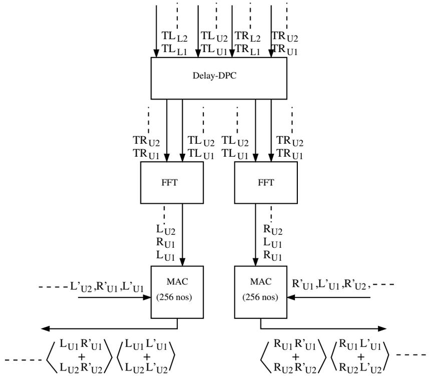
Figure 25.8: Signal flow in the GMRT correlator in the Polar Mode. Signal names preceded by a *T* indicate time series and angular brackets denote time average. See the caption of Figure 25.6 for other details.
