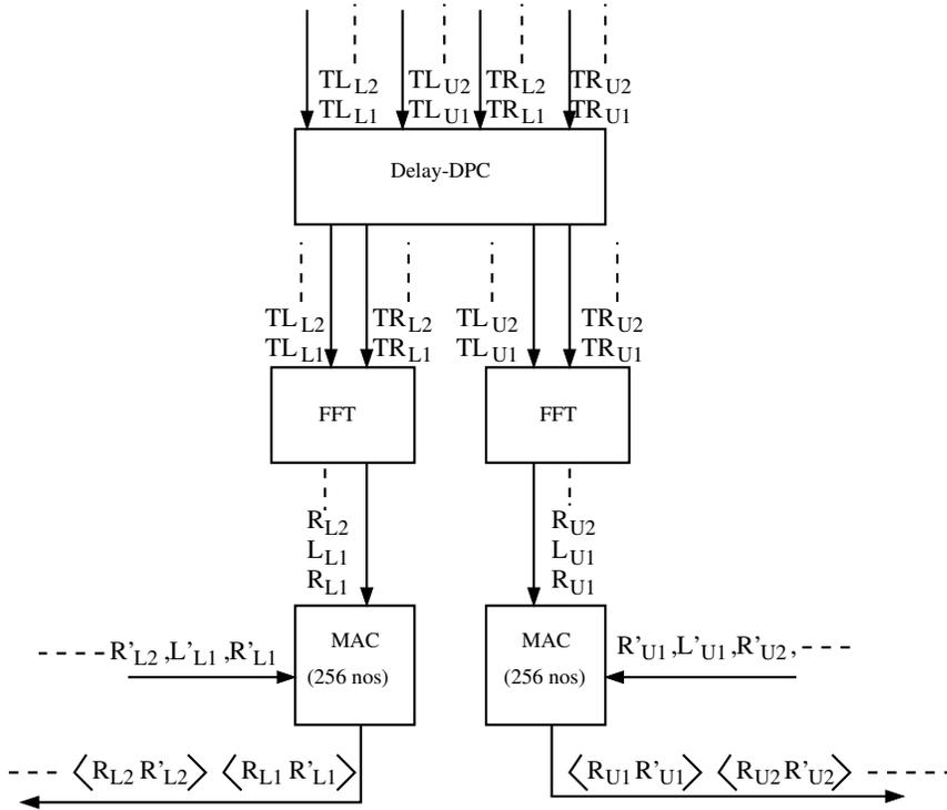
Figure 25.6: The signal flow in the GMRT correlator for the Non-Polar mode. Signal names preceding with a  $T$  indicate time series and angular brackets denote time average. Numeric subscripts indicate the sample number for time series data and the frequency channel number for spectral data.
