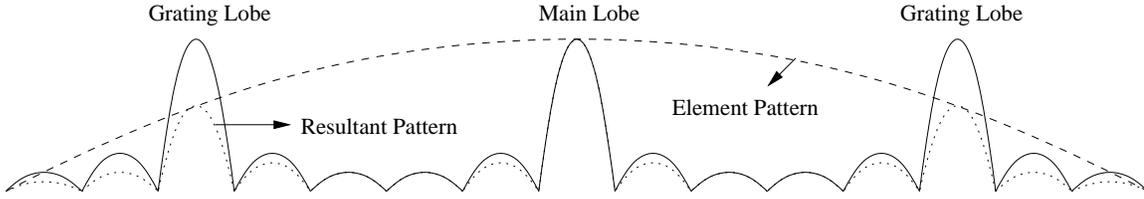
Figure 6.3: Grating lobes for an array of  $n$  identical elements. The solid line is the array pattern. The broad, dashed line curve is an example of the element pattern. The resultant of these two is shown as the dotted pattern.
