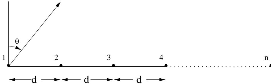
Figure 6.2: Geometry for the  $n$  element array
