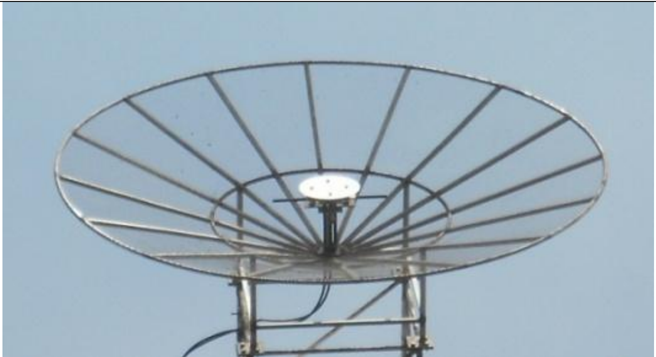
Figure 1: CDF 250-500 MHz mounted on antenna
