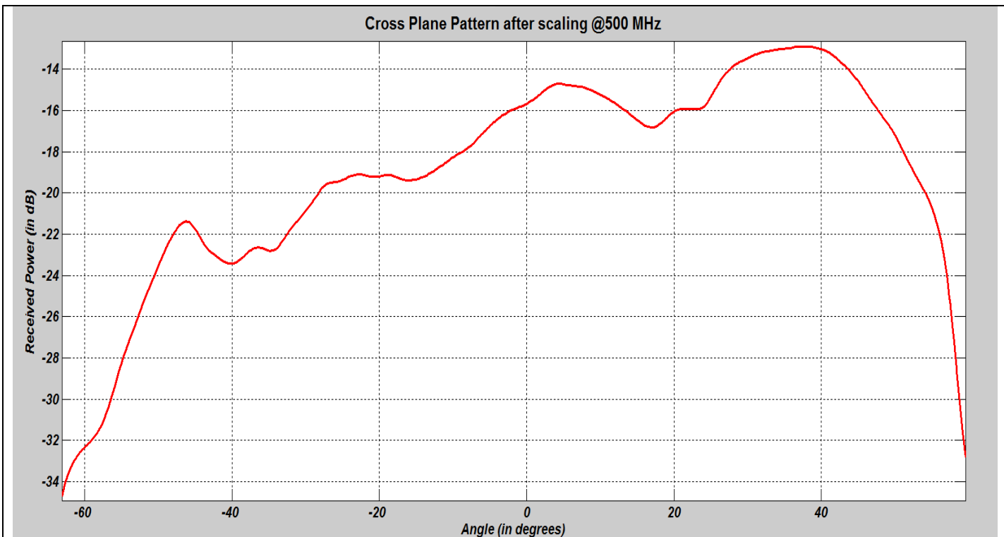
Figure 21: Cross-Polar pattern @ 500 MHz
