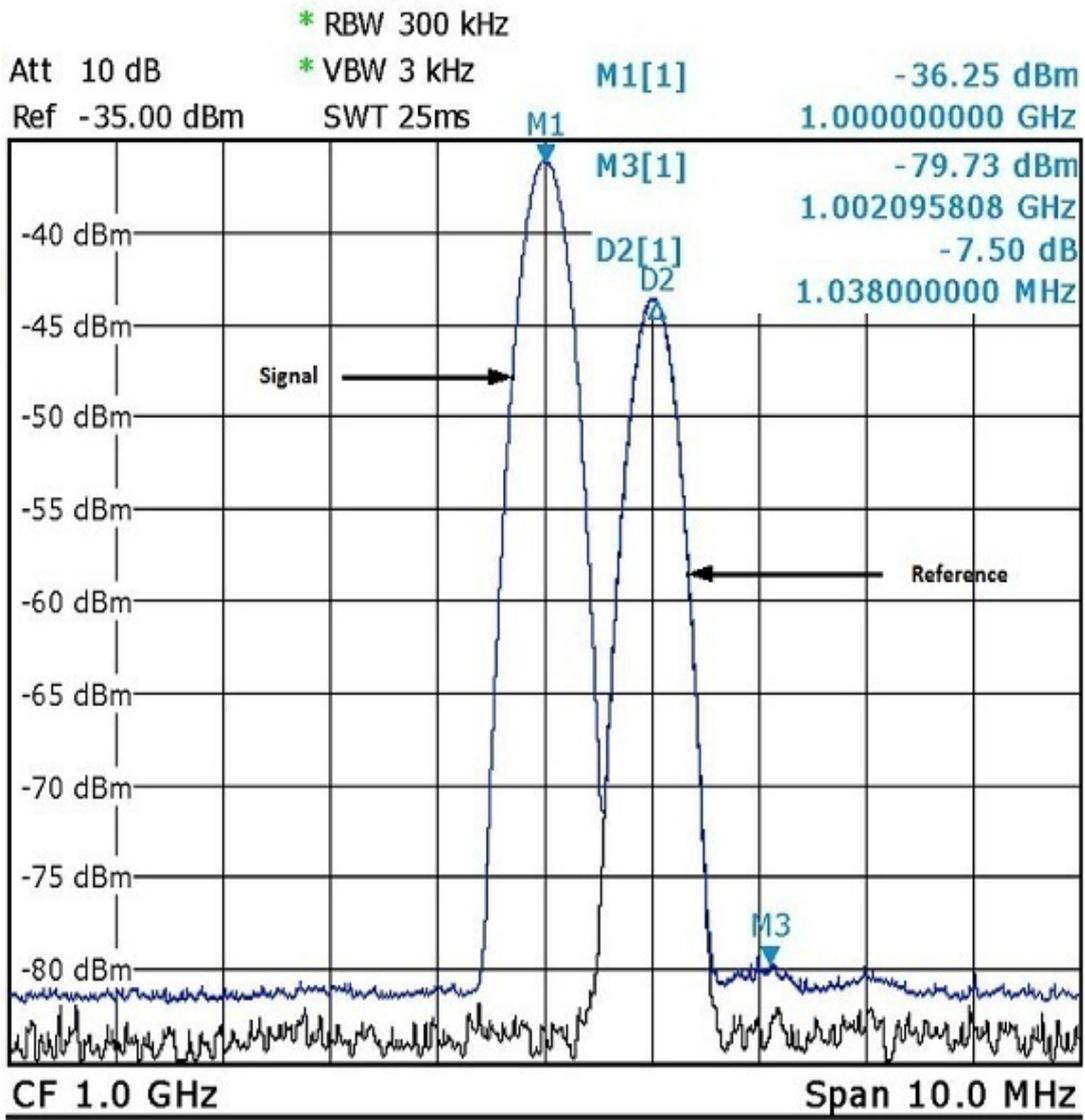
SNR measurement with respect to OFTx port at 1Ghz.
