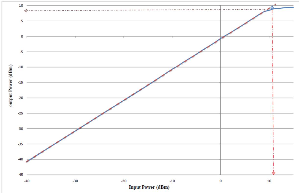
**Linearity performance of the integrated system with respect to IF Port.**
