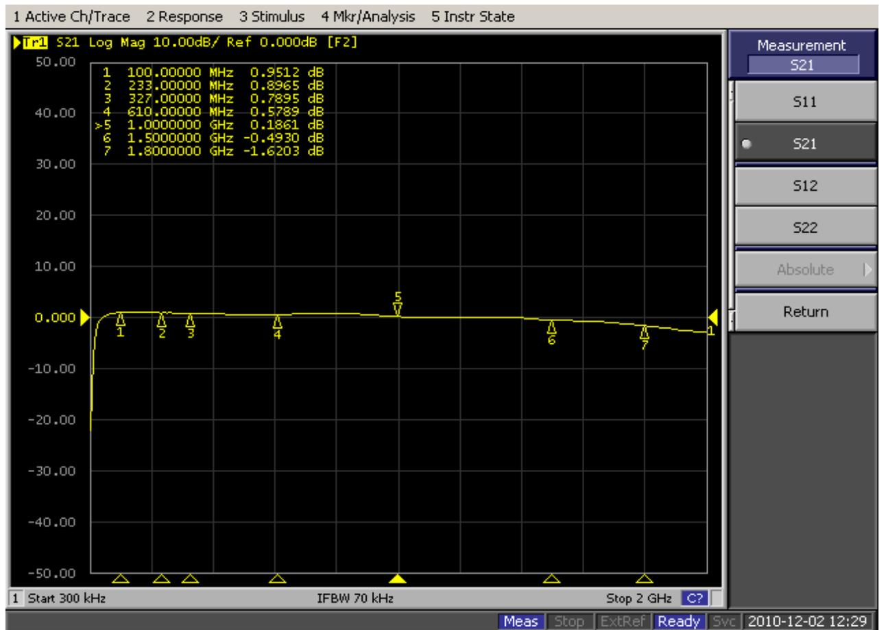
(Front End power levels to the IF input is maintained under +/- 1dB)
