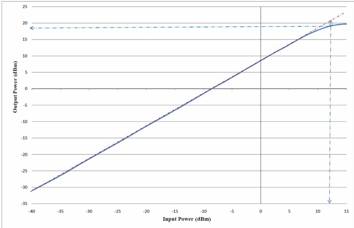
**Linearity performance of the integrated system with respect to OFTx Port.**
