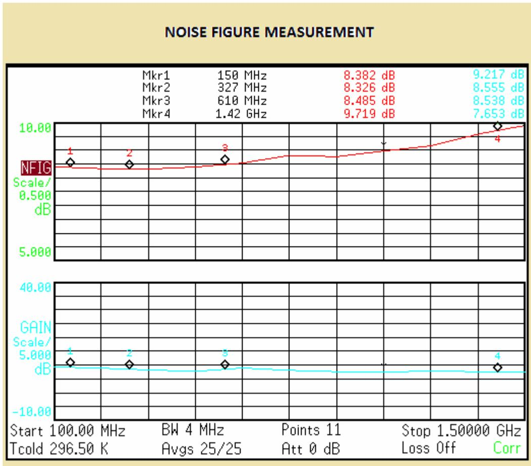
Noise Figure measurement with respect to OFTx port.
