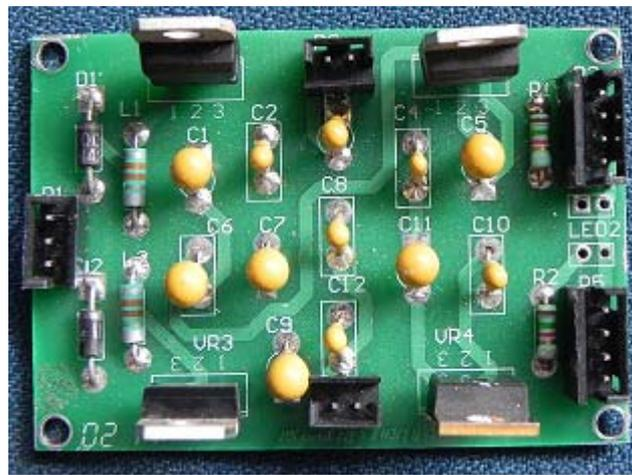
New DC Power Supply Card used in PIU
