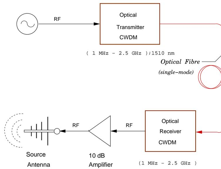
Fig. 3 Powering up the Source antenna – CWDM FO system.
