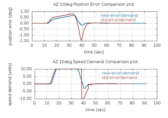
Case 4: Azimuth maximum tracking speed
