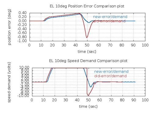
**Case 9: Elevation Maximum Tracking Speed Comparison**
