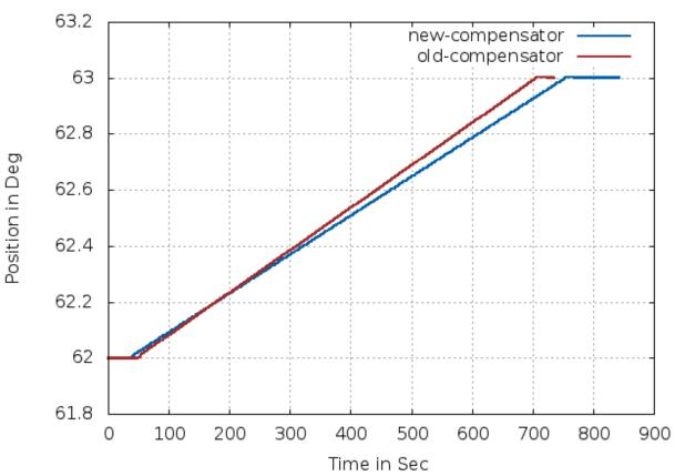
EL minimum tracking speed ramp response Comparison plot
