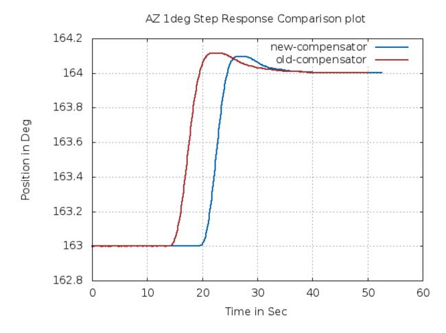
Time Domain Specification Comparison for one degree step
