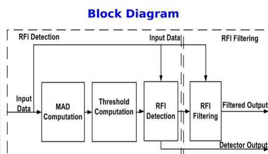
RFI mitigation block [3] was designed using MATLAB-Simulink and Xilinx System Generator and implemented on ROACH-1 FPGA board designed by CASPER collaboration (<https://casper.berkeley.edu/>).
